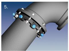
In large sizes (30-48 [and 54] inch), five or more repetitions may be required. The use of a torque-indicating wrench will facilitate this procedure.
