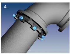
4.\* Push the gland toward the socket and center it around the pipe with the gland lip against the gasket. Insert bolts and hand tighten nuts. Make deflection after joint assembly but before tightening bolts.
