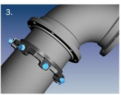
just prior to slipping the gasket onto the plain end for joint assembly. Place the gland on the plain end with lip extension toward the plain end, followed by the gasket.
